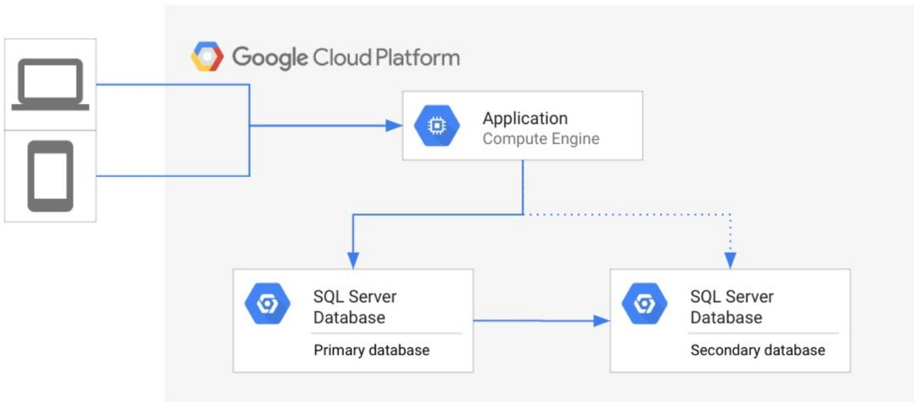
In the preceding diagram, an app accesses a primary database while a secondary database is standing by and mirrors the state of the primary database. Clients are accessing the app that runs on Google Cloud.
