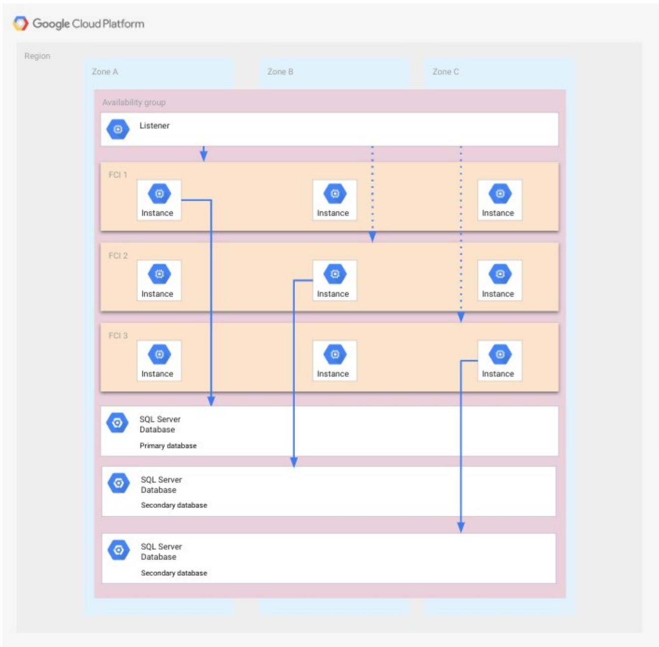
FCIs span all zones, and each FCI has one running SQL Server instance accessing the corresponding database. There are two more SQL Server instances that aren't running in each FCI that can be started up when a zone fails. The databases are shown across zones as each database uses the disks of all nodes in a given FCI. An app isn't shown for clarity.
